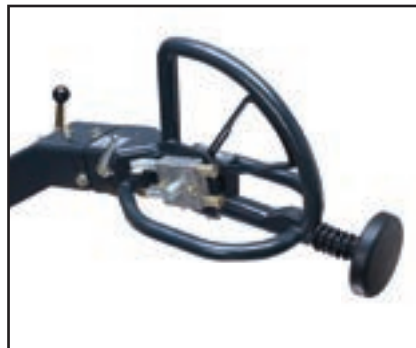
Safety steering handle with emergency stop for safe ergonomic operator control.
