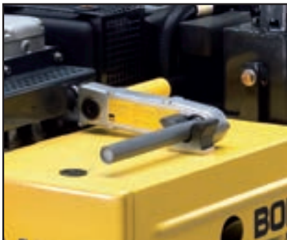
Standard electric start with back-up crank handle.
